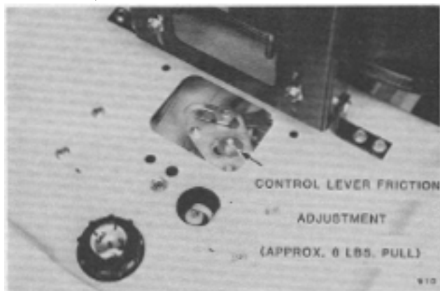
FIG. 12B. Late Model Friction Adjustment
