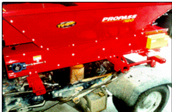
Figure 28: Lowering ProPass onto Workman
