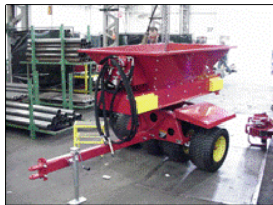
Figure 8: Lowering ProPass onto chassis
