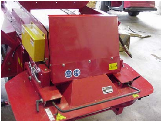
Figure 6: Front view of the hopper front guard
