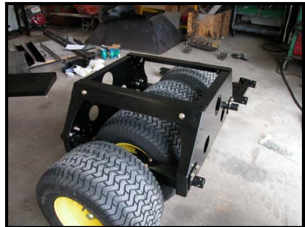
Figure 54: Cross Members Installed
