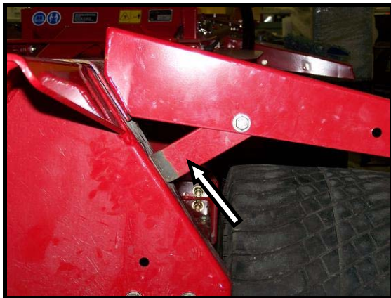
Figure 15: Fender Bracket Installed
