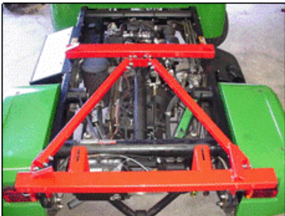
Figure 43: Installing braces on center cross member
