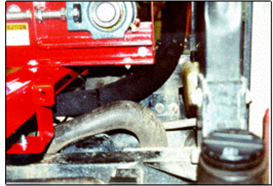
Figure 35: Route hydraulic hose away from other components
