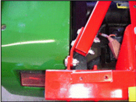
Figure 41: Installing brace tubes
