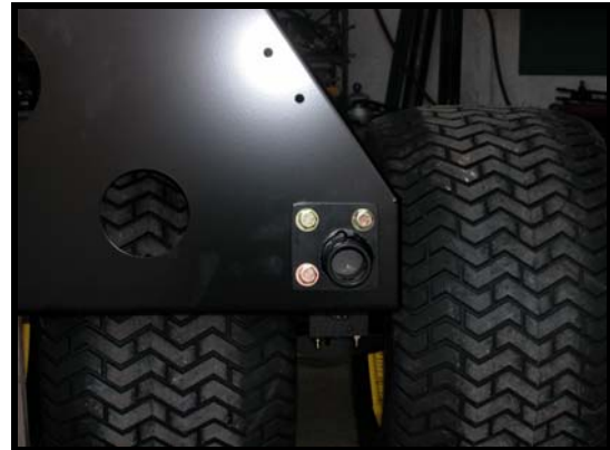
Figure 53: Jack Mount Installed
