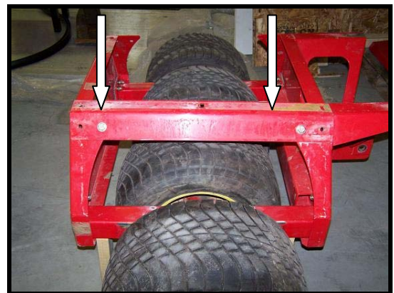
Figure 13: Only Use Inner Bolt Holes
