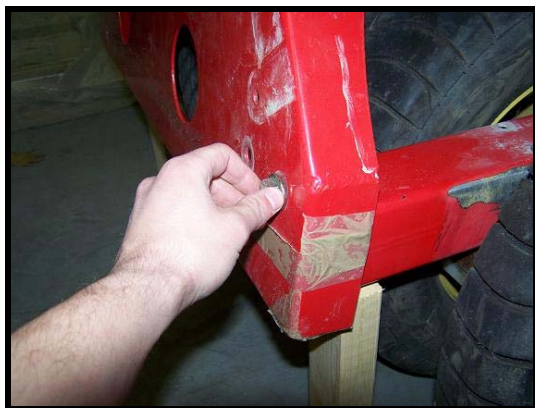
Figure 11: Finger Tighten Bolts
