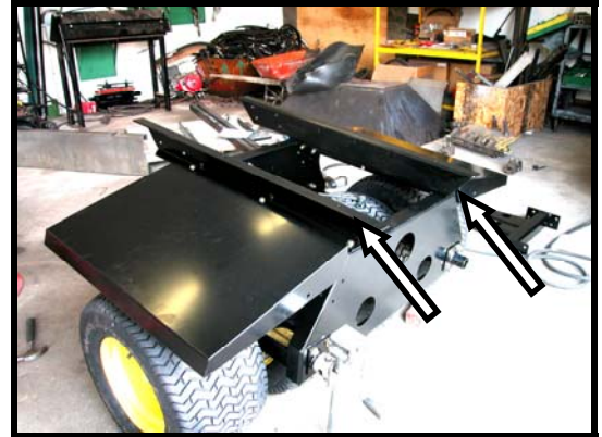
Figure 57: Side Rails Installed
