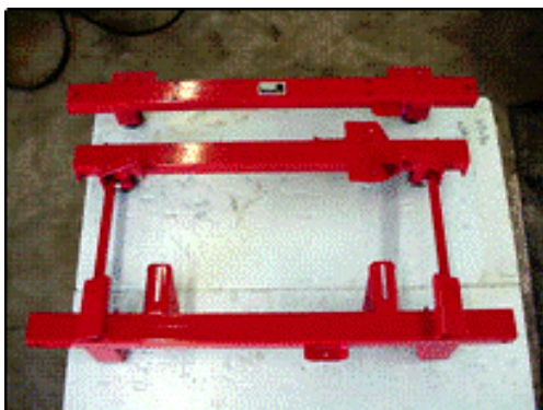
Figure 24: Installing center cross member
