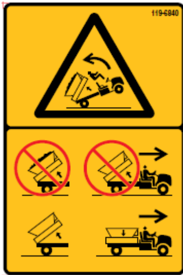
119-6840: Tipping hazard Lower hopper before driving
