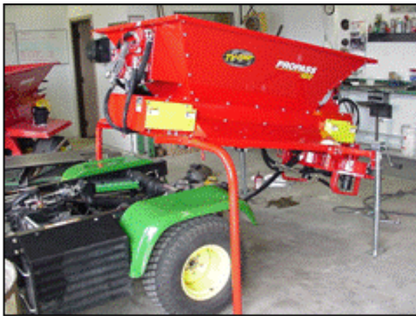
Figure 7: Installing the ProPass onto the work vehicle (or uninstalling it onto the storage stand)
