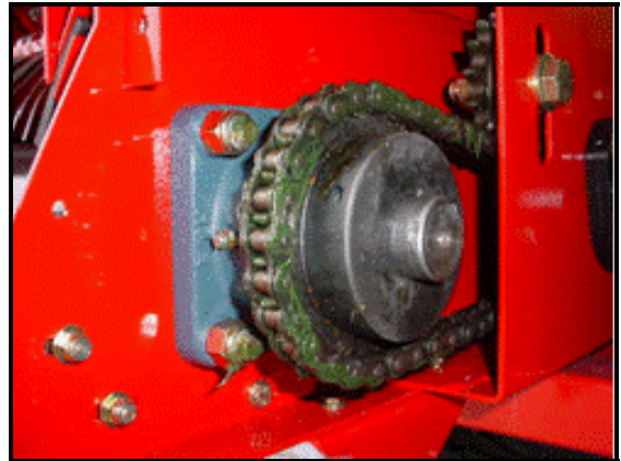
Figure 21: Grease fitting on Base Model (one at left rear, one at right rear)
