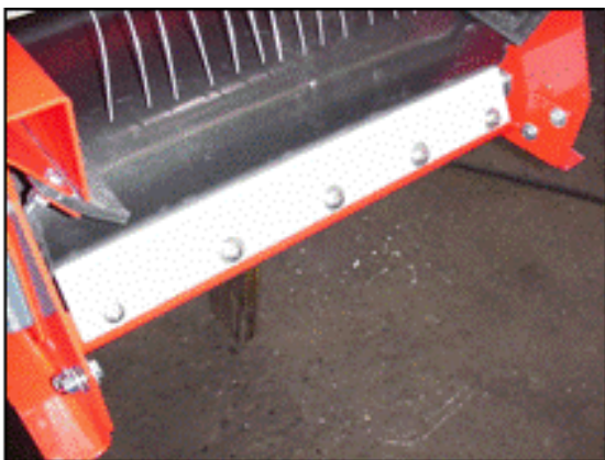
Figure 23: Belt cleaning scraper assembly
