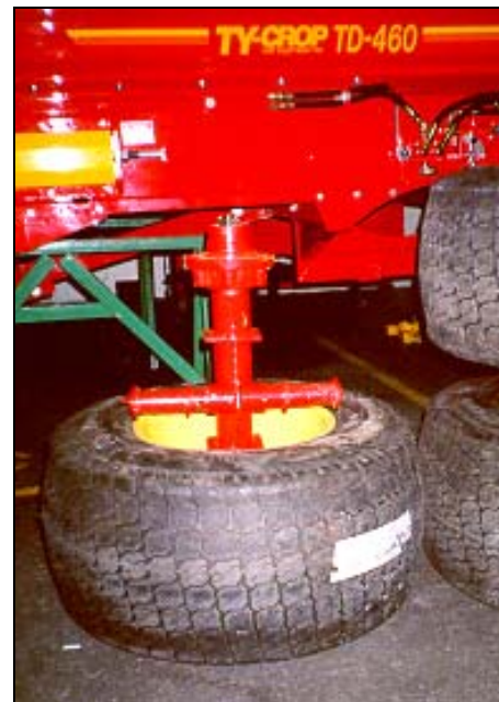
Figure 55: Flip tire and axle assemblies on end
