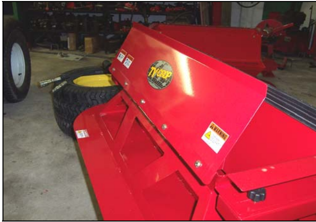
Figure 18: Install hopper front guard
