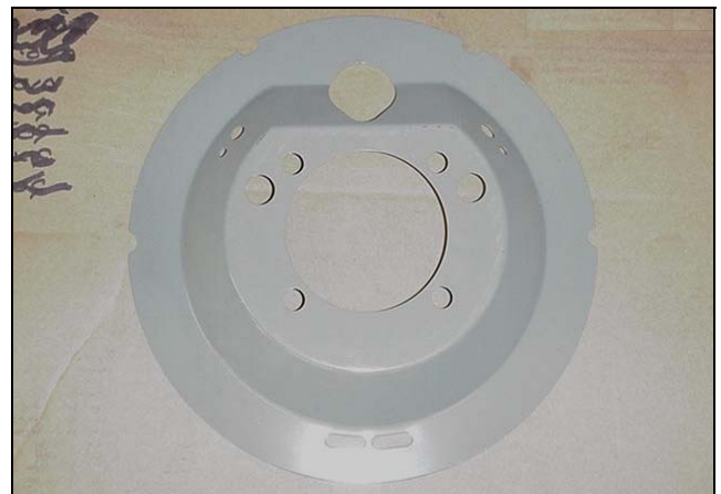
Figure 58: Install dust cover onto axle
