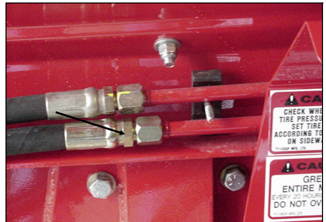
Figure 34: Install end of Item 8 hose to open hard line
