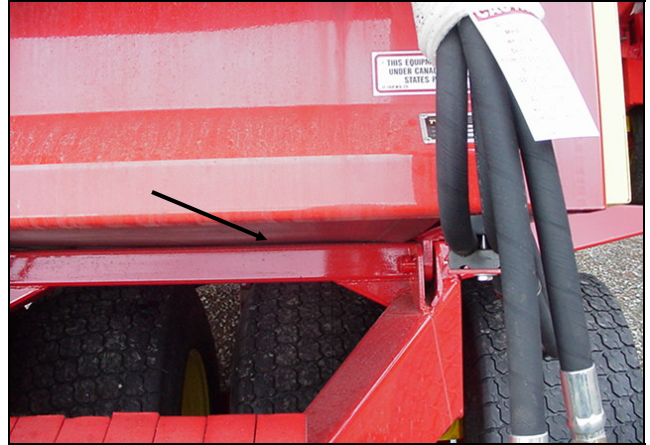
Figure 74: Attach connector bracket
