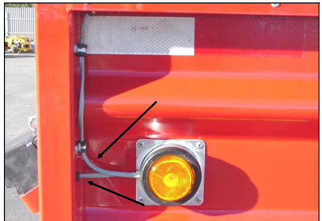
Figure 75: Wire front marker light
