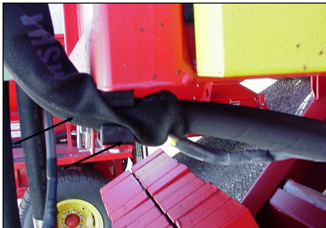
Figure 40: Slide sheath to hydraulic hose attachment; attach hydraulic hoses
