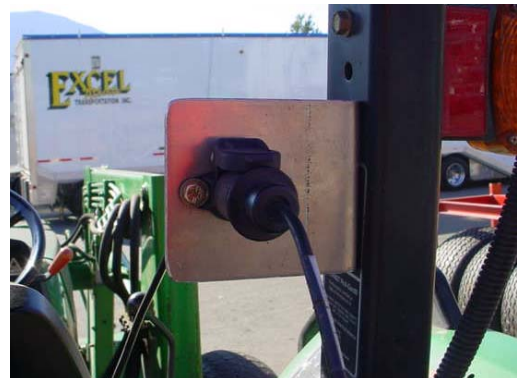
Figure 47: Attach SH Battery Harness to Solenoid Harness
