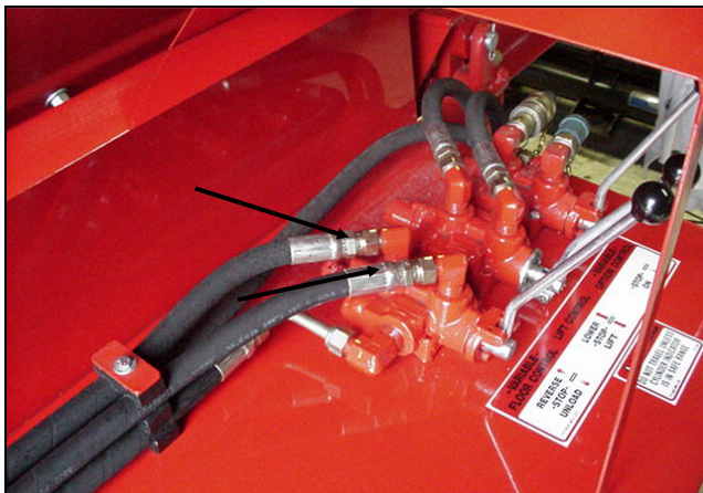
Figure 29: Remove and discard far hydraulic hose
