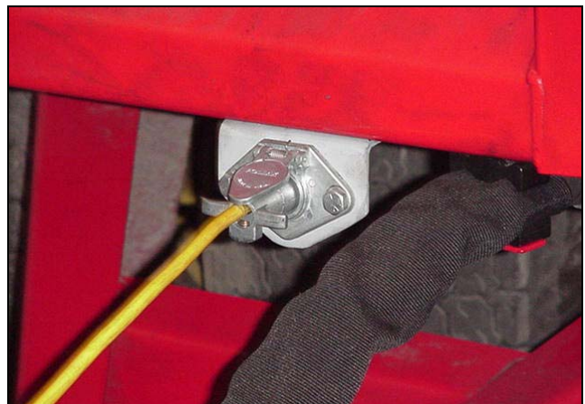
Figure 11: Plug in on/off pendant switch on SH Models
