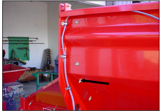
Figure 70: Remove bolt for rear taillight bracket
