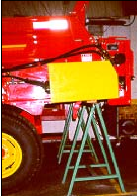
Figure 53: Raise and support the MH-400
