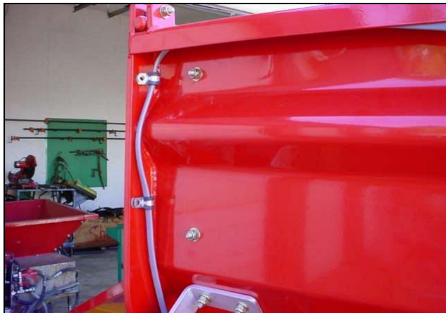
Figure 76: Wire rear taillight
