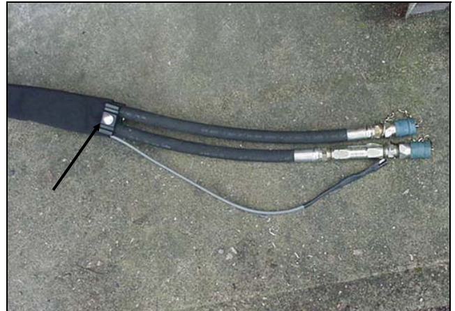
Figure 41: Pull hoses straight and tighten
