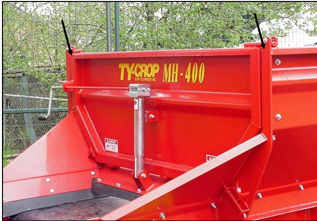
Figure 8: Remove bolts and nuts from rear gate
