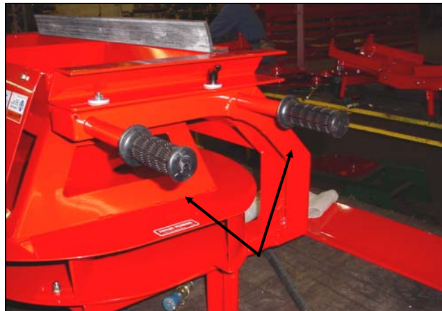
Figure 16: Install Twin Spinner handles
