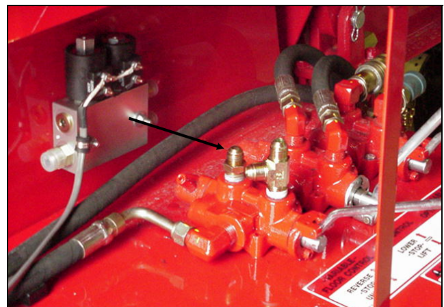
Figure 31 Install connector fitting to inside valve port
