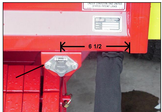
Figure 42: Attach mounting bracket for electric socket
