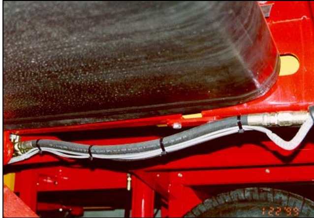
Figure 63: Run wire along hydraulic hoses to 7-prong plug
