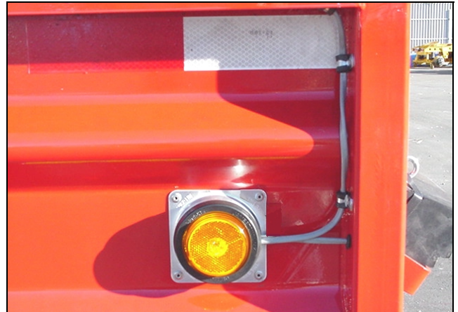
Figure 77: Wire side marker light
