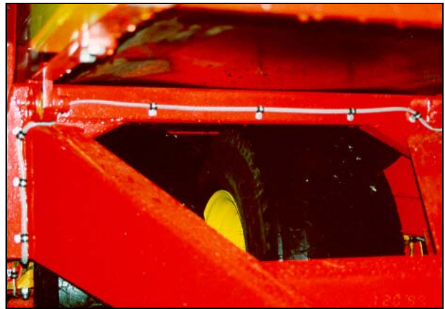
Figure 62: Run wires for left side up and under pivot point of MH-400
