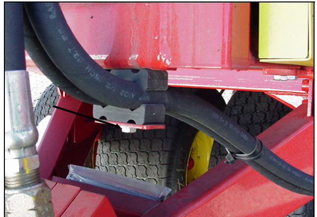
Figure 38: Remove hydraulic hose clamp
