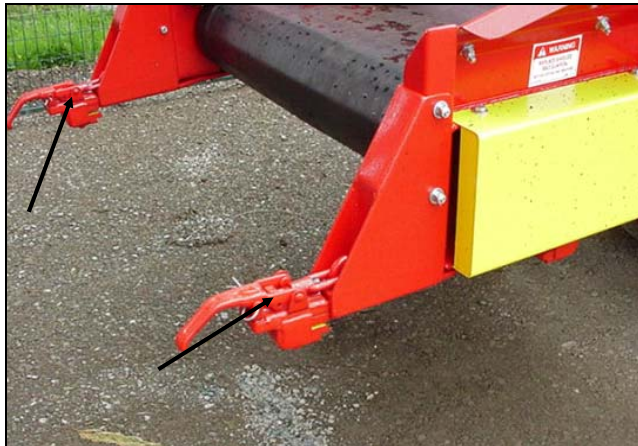
Figure 4: Install option attachment clamps
