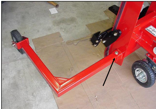
Figure 12: Install legs on option caddy
