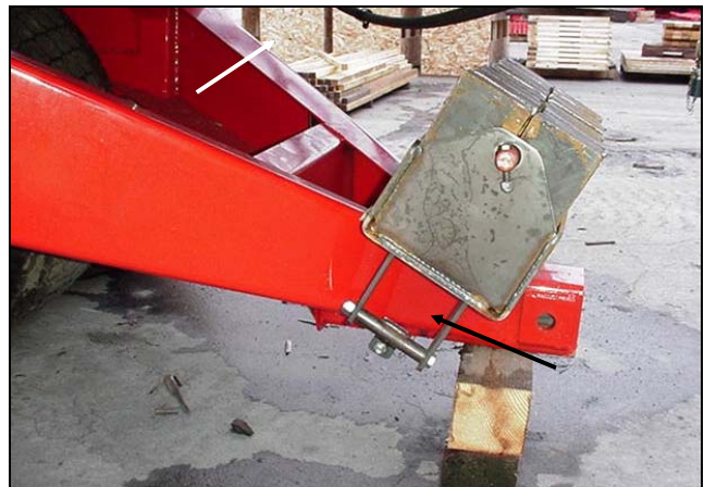
Figure 3: Remove bolts from weight case mounting bracket
