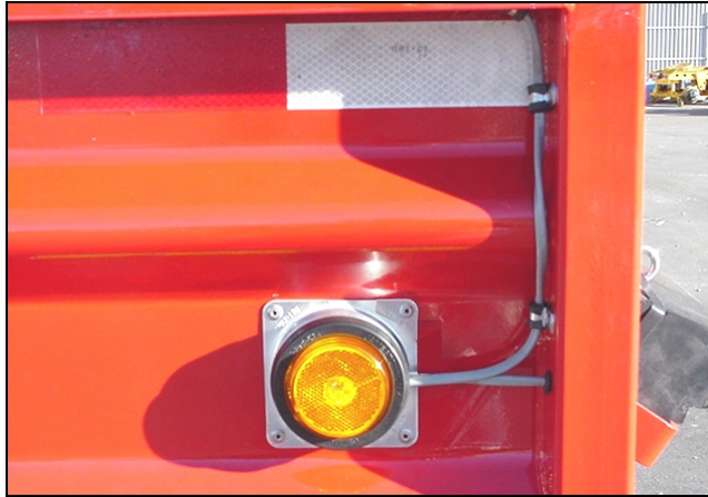
Figure 69: Position front side yellow marker light
