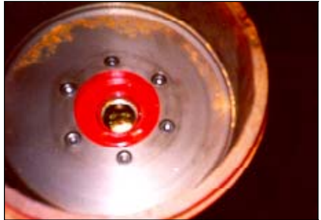
Figure 57: Mount hub assembly onto drum
