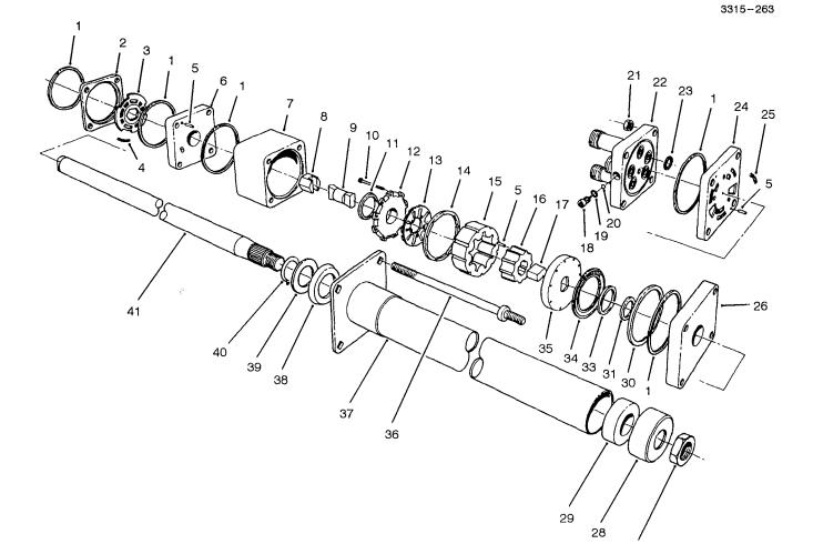
POWER STEERING VALVE ASSEMBLY NO. 63-9250
