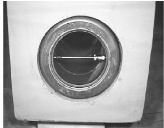
Figure 04-10 Measuring the Lower Chuck Bushing or Insert for Wear
