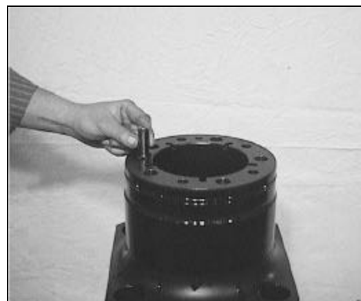
Figure 08-35: Insert Cylinder Centering Pin
