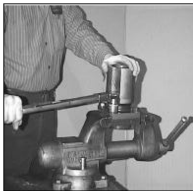
Figure 06-05: Torque Accumulator Shell Bolts MES 150
