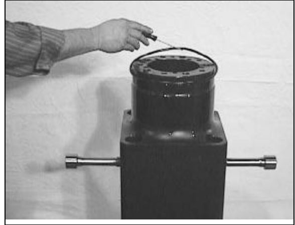
Figure 08-33: Install Cylinder O-ring
