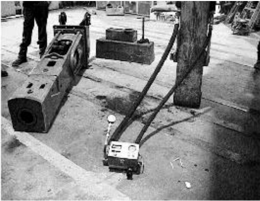
Figure 01-01: Testing Excavator Circuit Flow and Pressure
