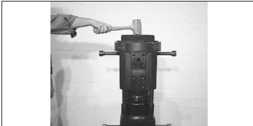
Figure 08-44: Using a Dead Blow Hammer to Drive Head down
