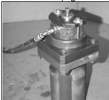
Figure 06-22: Installation of Inflation Body MES 150
