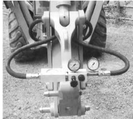
Figure 01-02: Testing Tractor Loader Backhoe Circuit Flow and Pressure
