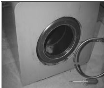
Figure 04-11: Remove Insert Snap Ring
