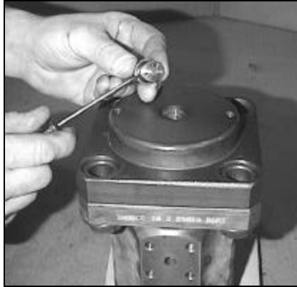
Figure 06-02: Loosen Inflation Screw Carefully MES 150
