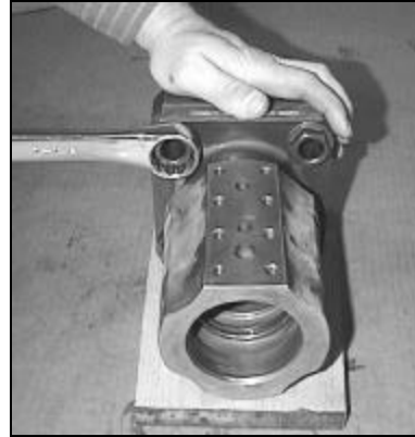
Figure 06-03: Remove Accumulator Shell Bolts MES 150
