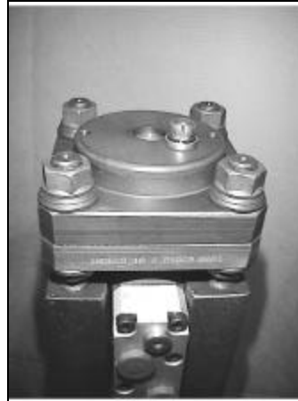
Figure 06-06: Install and Torque Accumulator MES 150
