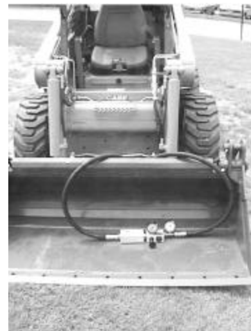
Figure 01-04: Testing Skidsteer Loaders Circuit Flow and Pressure
