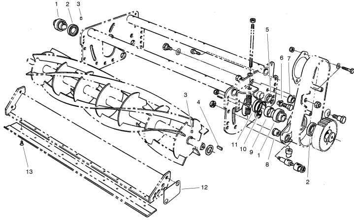
Note: For cutting units with serial number 39999 and down use flange bushing p/n 72-0430 Qty. (2). Not supplied with this kit.
