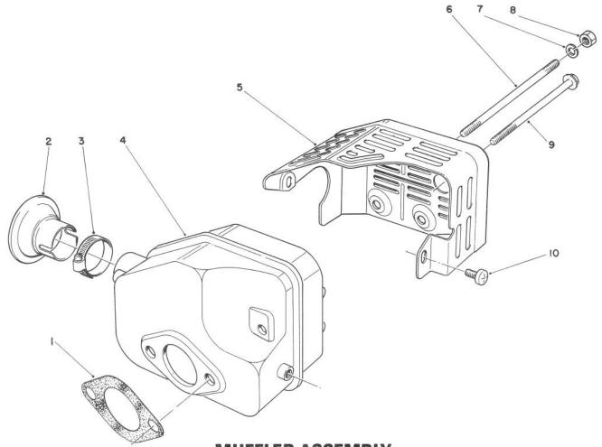
MUFFLER ASSEMBLY (Engine No. 47PF5) (Engine No. 47PG6)
