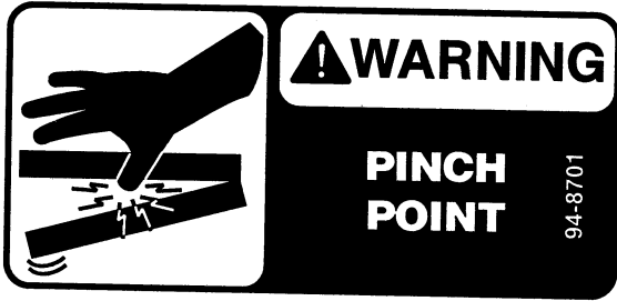
Part No. 94-8701 Located on Center Section Ends and on Boom Extension Hoods near Actuator Link.
