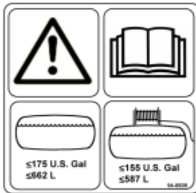
Part No. 94-8609 WORKMAN® Vehicle only - Located on either side of the rear Spray Tank Band and Hose Reel, if equipped with one. Enclosed Boom - Located on rear left side of Center Section.
