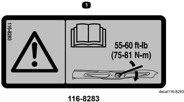
1. Warning—read the *Operator's Manual* for instructions on torquing the blade bolt/nut to 75 to 81 N·m (55 to 60 ft-lb).
