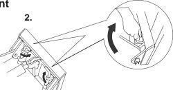
3. Ensure that the pins are engaged in the holes in the attachment mounting plate.
