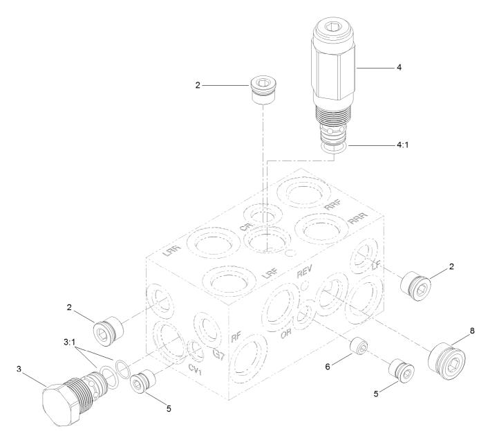
Four Wheel Drive Manifold Assembly No. 108-1825
