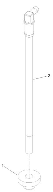
Fuel Pickup with Screen Kit Assembly No. 161-6806
