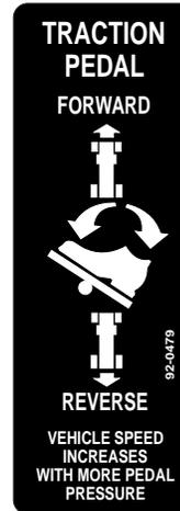
Part No. 92-0479: Located on Floorboard, Right of Traction Pedal.
