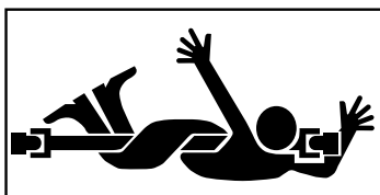
WHOLE BODY ENTANGLEMENT, IMPLEMENT INPUT DRIVE LINE
