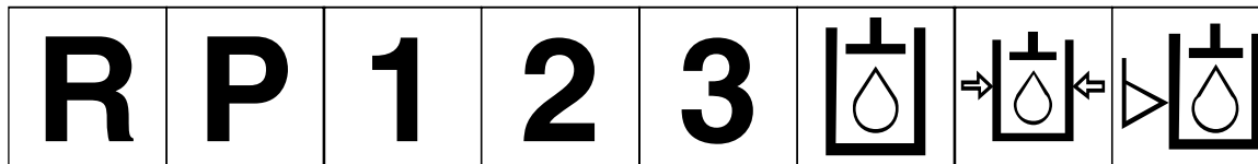
Reverse Park First gear Second gear Third gear (other #'s may be used until the maximum # of forward gears is reached.) Hydraulic oil Hydraulic oil pressure Hydraulic oil level
