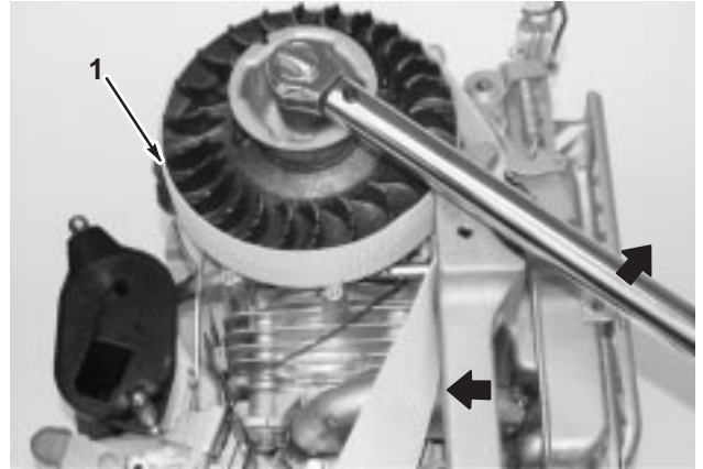
Fig. 13 – Removing Flywheel Nut
