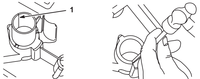
Fig. 143 – Locating and Staking Bearing
