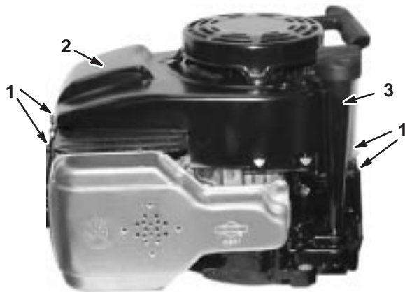
Fig. 70 – Removing Oil Fill Tube
