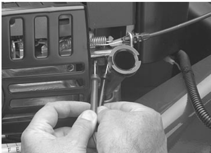
Fig. 95 – Checking the Brake Switch
