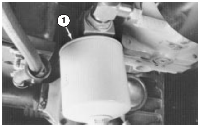
Figure 60 1. Hydraulic oil filter
