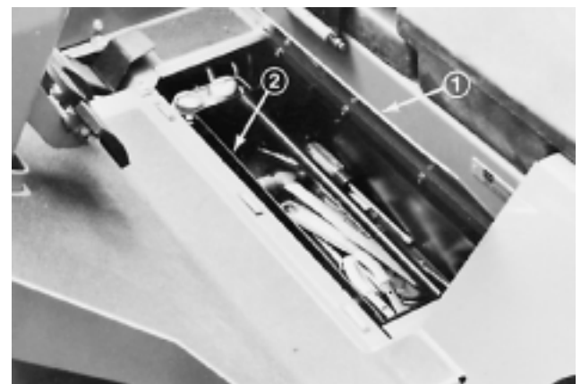
Figure 20 1. Hinged Floor Plate 2. Removable Tool Tray
