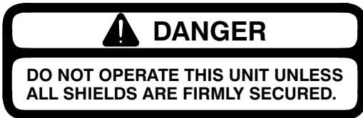
ON LEFT, CENTER AND RIGHT SIDES OF DECK, UNDER SHIELDS (Part No. 67-5360) (Part No. 93-7273 for CE)
